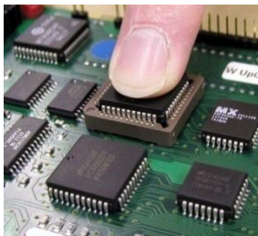
Carefully press the chip into the cap.
