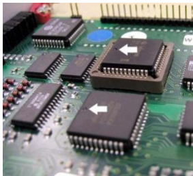
Insertion of the chip to the cap. ATTENTION! Please watch the chip orientation – it must be the identical with that of the other chips!
